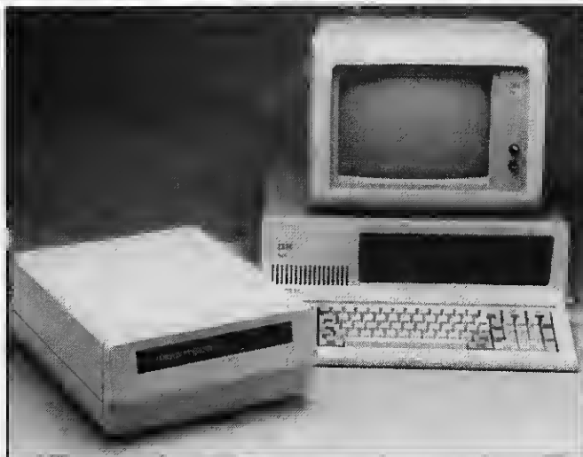
The Corvus Constellation, a local network based on a Corvus hard disk drive, can now be used to link IBM Personal Computers together, sharing mass data storage (hard disks) and other expensive peripheral devices.
